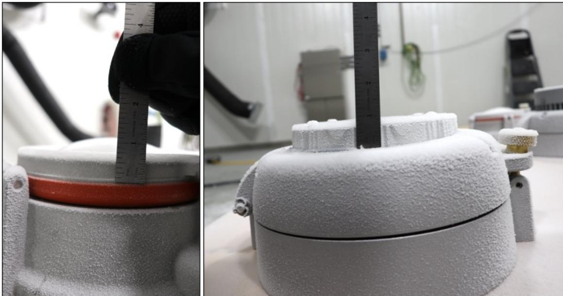
**Figure 5. Light fixtures with 1/4-inch accumulation of ice**
