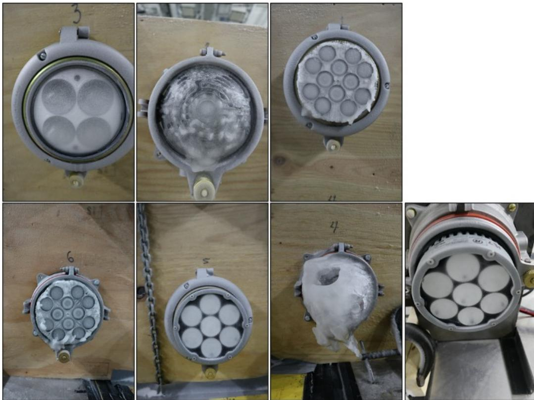
**Figure 15. Close-up view of the accumulation of snow and ice on light fixtures after Trial 1**
