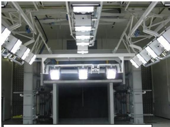
Solar array showing front illumination (9.3m<sup>2</sup> nozzle)
