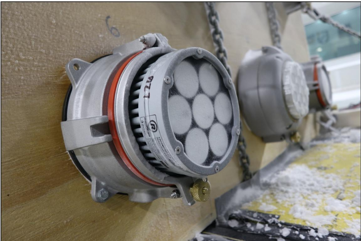
**Figure 46. LED sample after Trial 2 (non-powered sample)**
