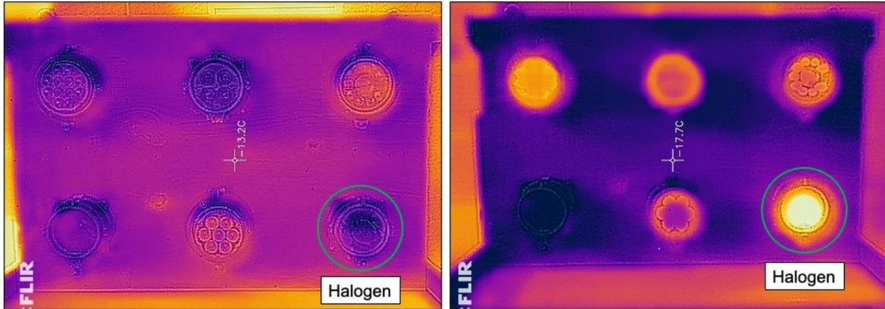
**Figure 2. Thermal image of preliminary temperature testing**
