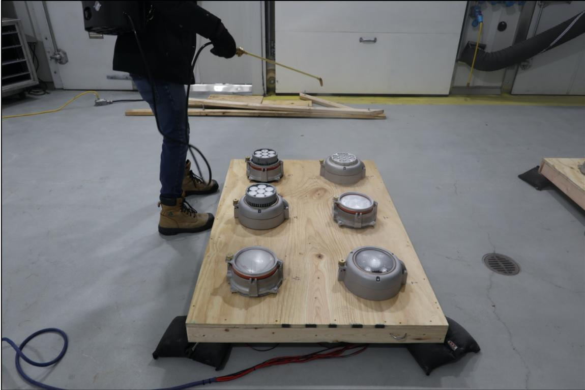
**Figure 52. Early stages of the water spraying process**
