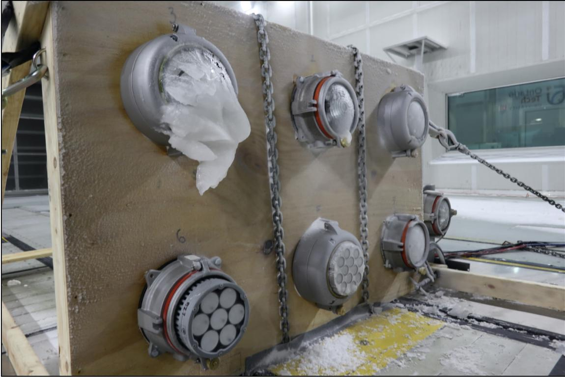
**Figure 41. Light fixtures after Trial 2**
