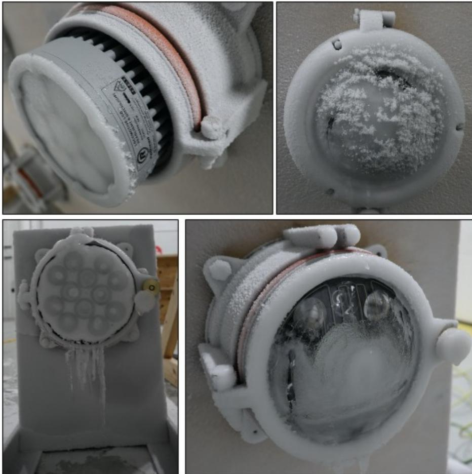
**Figure 10. LED light fixtures after 30 minutes of operation at -20 °C**
