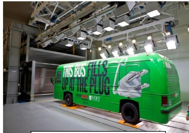
Solar array arranged for a bus (13m<sup>2</sup> nozzle and 22m<sup>2</sup> canopy)
