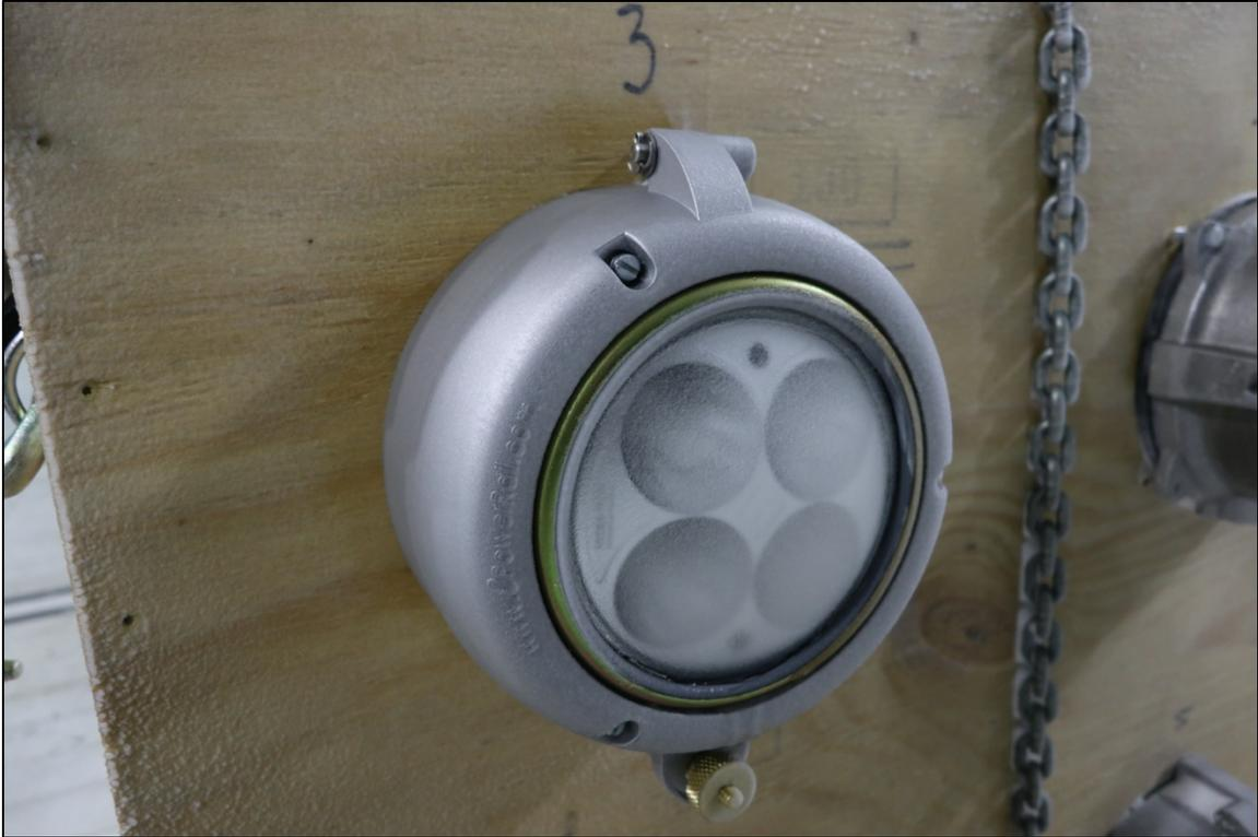
**Figure 36. LED sample after Trial 1**
