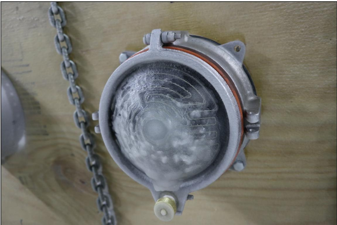
**Figure 35. LED sample after Trial 1**
